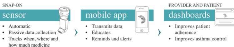
FIGURE 1: The Propeller Health sensor attaches to a metered-dose inhaler (MDI) canister, and pairs with smartphone and web applications that present visualized data and trends
